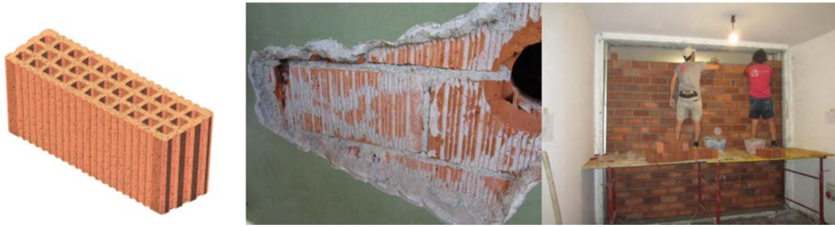
Figure 1: From left to right: the brick typology, the wall where the core sampler was used (showing the brick typology) and the installation of the wall in laboratory.
