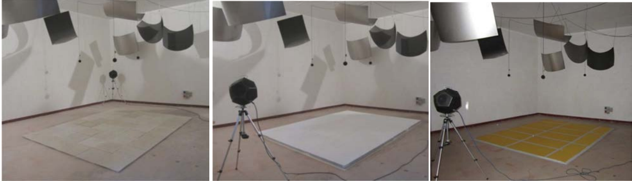
Figure 6: From the left to right: laboratory measurements of sound absorption in reverberant room for systems A, B (with finish) and C.
